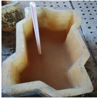
Fig .12 Dented Type-A Interlocking Paver Block Mold with Straw.
