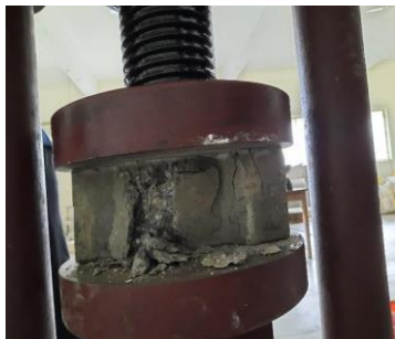
Fig.17 Mode of Failure of Pervious Paver Blocks
