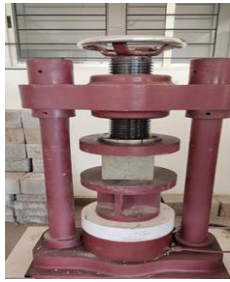
Fig .16 Compressive Strength Test of 100X100X100 mm Specimen
