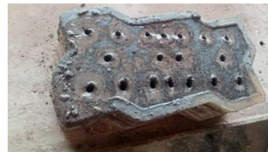
Fig .15 Paver Block kept for Air Curing.
